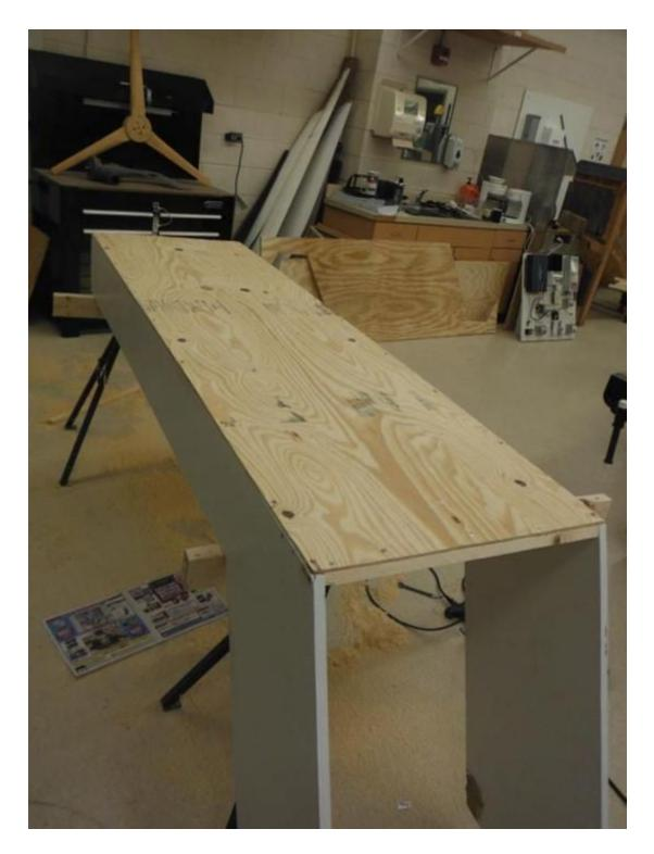
Remember that sheet of quarter-inch exterior grade plywood in the materials list? Cut a 24-inch-wide piece from it that's the same length as the bottom of the collector box. In this design, the length is 6 feet and 11 inches, but the dimension will be different if you changed the angle of the collector to make a solar dehydrator specific to your latitude.
