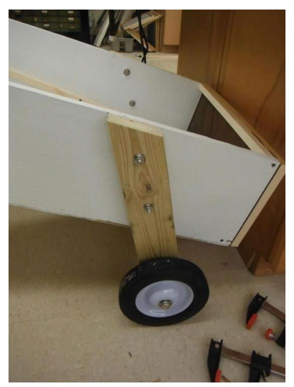
It's time to get the solar dehydrator standing on its own four legs. These plans call for two front and two rear legs made from pressure-treated 2-by-4s, and attached to the dehydrator using two 3/8-inch-diameter-by-3-inch-long bolts, nuts and washers each. Install the two front
