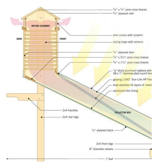
As you can see in the detailed drawing, the design includes a long, angled wooden box covered with clear plastic glazing and an open bottom end for air intake. Inside, the box holds diagonal layers of black metal screen. The vertical drying chamber on top has a back door to access food-drying trays inside.
