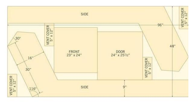
Most of the wood required for these solar food dehydrator plans can be cut from a single 4-by-8-foot sheet of three-quarters-inch-thick exterior-grade plywood. Measure and mark the plywood using the cutting diagram (above) as your guide. Note that the dryer sides are cut in a single piece so there's no joint between the collector box and the drying chamber. You should mark the dehydrator's sides on opposite edges of the plywood sheet to leave space in the center for the other pieces you'll need.
