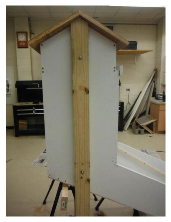
The solar dehydrator's roof is made of two pieces of three-quarters-inch plywood, preferably scraps you have lying around in your workshop. You also can create three-quarters-inch plywood by gluing together several pieces of the one-quarter-inch plywood left over from cutting the front of the dehydrator. The roof is made up of two 12-by-30-inch pieces, with
